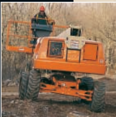
Oscillating Axle for Tough Travel
